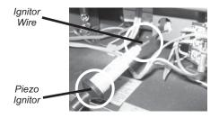
Disconnect the ignitor wire from the Piezo Ignitor and connect it to the DC Sparker.
